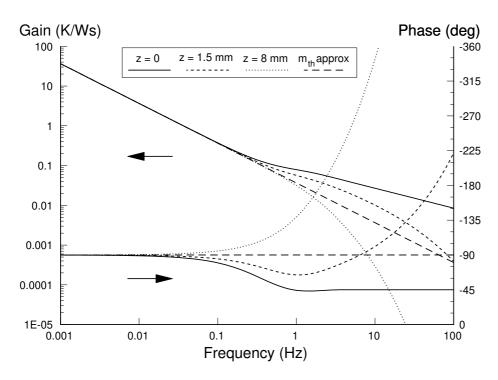
**Figure 20.2** Gain and phase transfer function of thermal diffusion in an 8mm thick plate of 6061 aluminum, for sensors mounted at z=1.5 mm and z=8 mm, compared with the thermal mass approximation.
