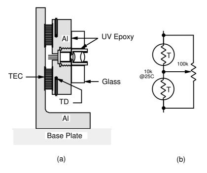
**Figure 20.7** Cancellation of temperature gradient by common centroid design. (a) Thermistors placed symmetrically about diode laser. (b) Series connection gives  $T_{avg} \approx T_{laser}$ , allows vernier adjustment.
