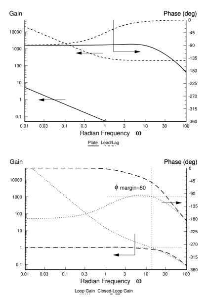
**Figure 20.9** Bode plot of the 8-mm thick aluminum plate of Figure 20.2, with the temperature sensor at *z*=3mm, using lead-lag compensation. The unity gain bandwidth is over 2 Hz.
