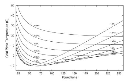
**Figure 20.6** Choosing the right TEC for a given  $\dot{Q}_{\text{load}}$  and  $\Theta_{\text{SA}}$ . Here the cold plate temperature bottoms out at about -10° C over a fairly broad TEC size range of 50–75 junctions. ( $T_A$ =25° C)
