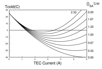
**Figure 20.5** Designing a TE cooler system using a passive heat sink: cold plate temperature *vs*. I and heat sink thermal resistance  $\theta_{SA}$ . ( $T_A=25^{\circ}$  C)
